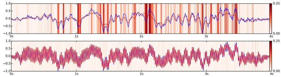
**Fig. 1.** Input (blue) and reconstruction (red) for 4s of EEG data sampled at 100Hz (top) / 400Hz (bottom). Background color indicates the squared sample error (right scale).
