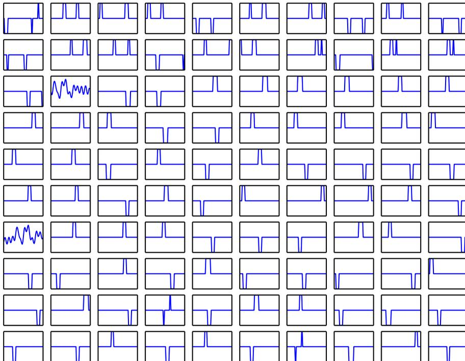
**Fig. 2.** Top 100 input segments (200ms at 400Hz) with highest reconstruction error and clearly visible artifacts.
